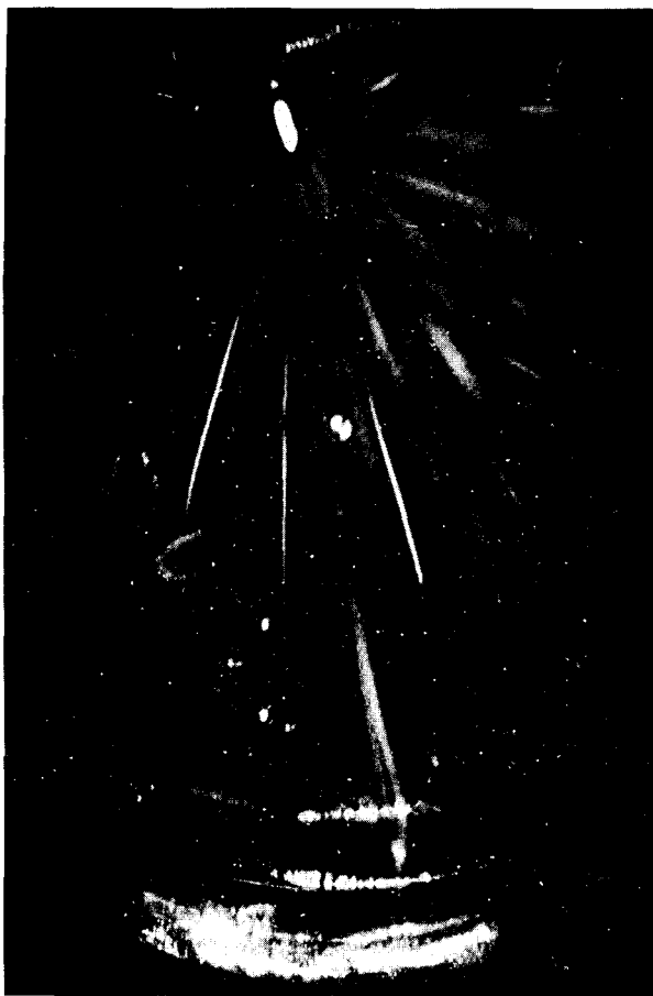
9. One of the first photographs to show the tracks of subatomic particles in a cloud chamber. The picture was taken by the cloud chamber's inventor, English physicist C. T. R. Wilson, at the Cavendish Laboratory in Cambridge in 1911. The tracks are due to alpha particles emitted by a small amount of radium on the top of a metal tongue inserted into the cloud chamber. As an electrically charged particle moves through the water vapour in a cloud chamber, it ionizes the gas, and water drops condense on the ions, thus producing a track of droplets where the particle has passed.
